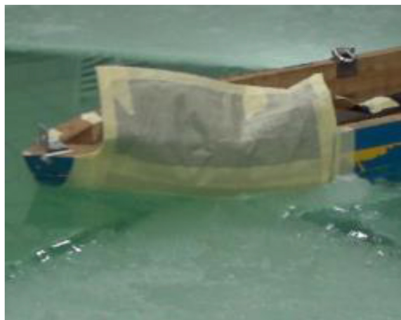
Fig. 9. Lab model test of Xuelong 2. Source: By authors.
