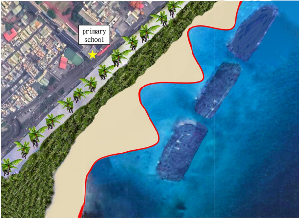
Fig. 15. New innovative submerged breakwaters combined with an artificial beach.
