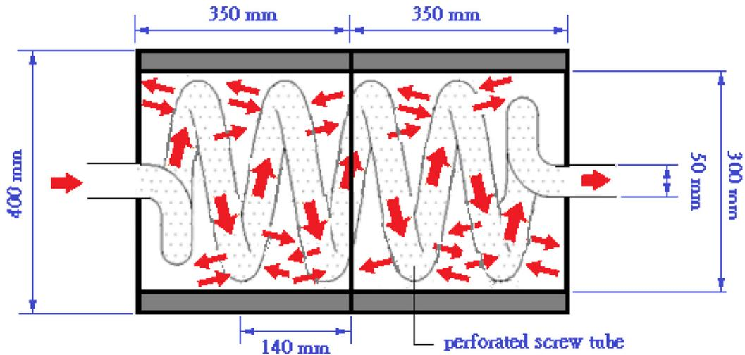
(b) Silencer B (a two-chamber design internally inserted with two screw and perforated tubes and one perforated tube).
