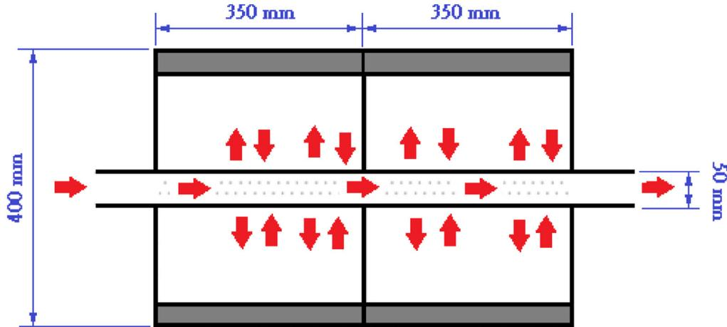
(a) Silencer A (a two-chamber design internally inserted with a straight and perforated tube)
