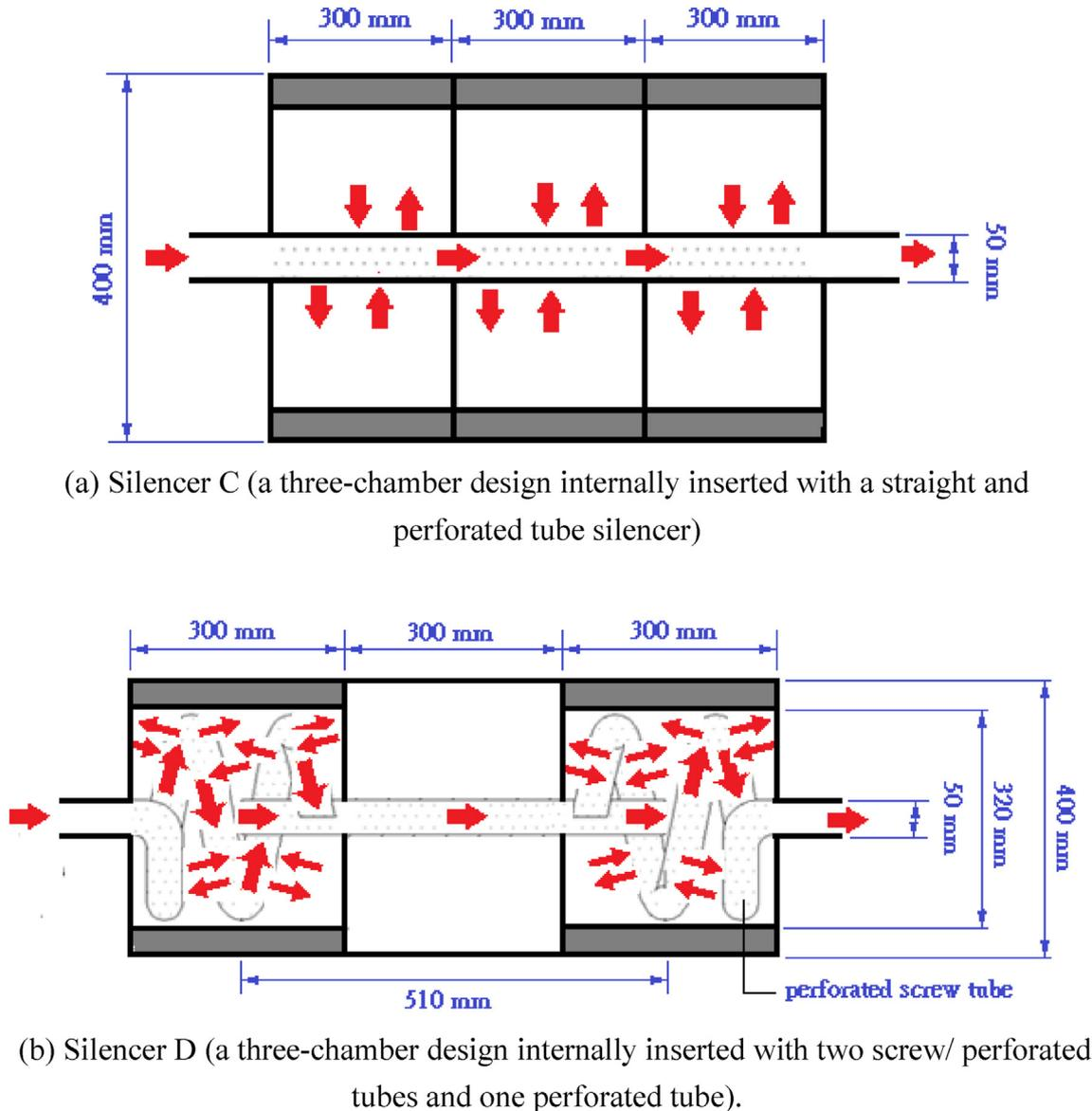
Fig. 2. Acoustical mechanisms of silencers C and D.
