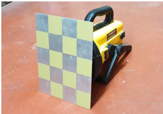
Fig. 3. Calibration target consisting of an aluminum board in a checkered pattern and a lamp.
