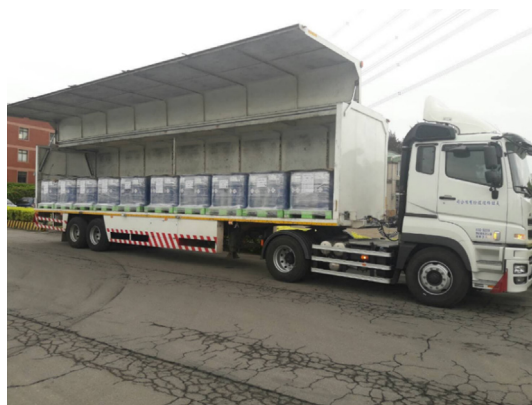
Fig. 1. A truck with a gross weight of 35 tons and a size of 20 pallets.
