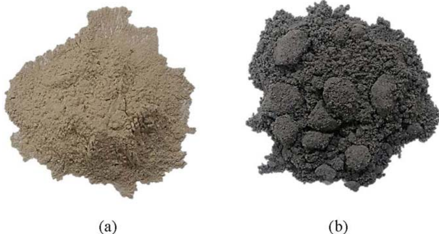
Fig. 1. CFBC ash appearance: (a) Type A (b) Type B.
