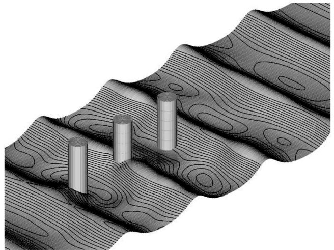
Fig. 13. Three dimensional perspective view of the elevation in presence of the three tandem cylinder array at t = 105 \text{ s } (kr = 1, \epsilon = 0.3, m = 0.9, \lambda = 6.14 S/r = 3) .
