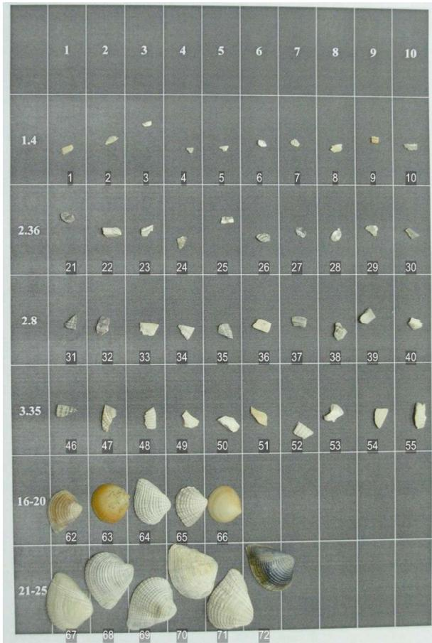
Fig. 4. Sample shell pieces used in the laboratory experiment. The numbers in the first column are the size (mm) in the bin. The number adjacent to each shell pieces is a unique ID used in the random process of location generation.
