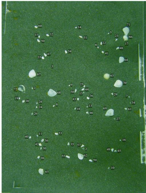
Fig. 6. Simulated seafloor covered with shell pieces for the laboratory experiment. Each shell piece is labeled with the number assigned in Figs. 4 and 5.
