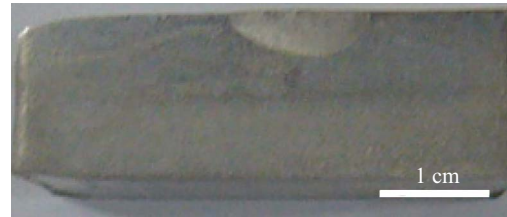
Fig. 7. The x-x' section view of heated workpiece with traveling speed 1 mm/s under incident power 6.8 kw applied.
