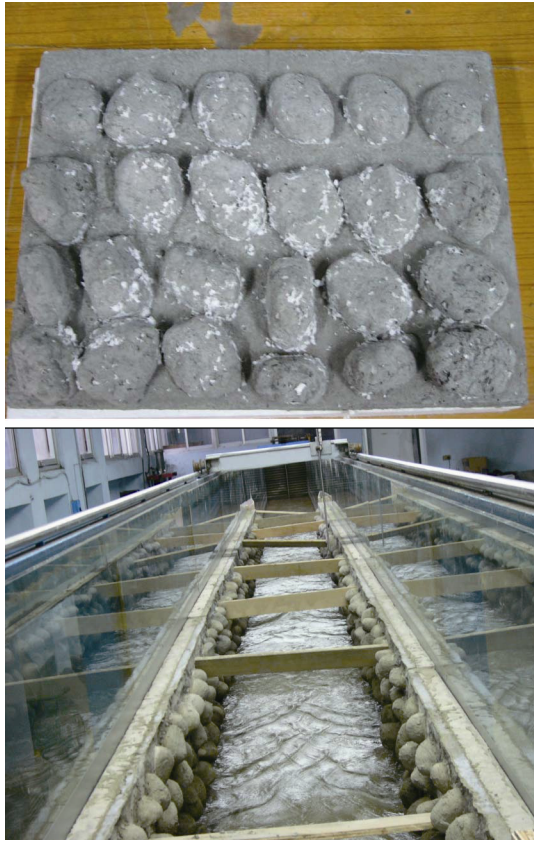
Fig. 1. Precast ecological concrete block model and its test in the flume.
