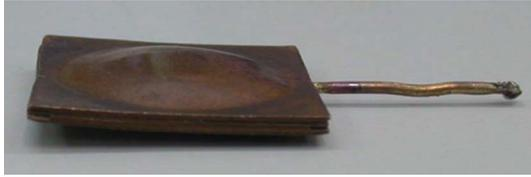
Fig. 1. Deformation of vapor chamber.
