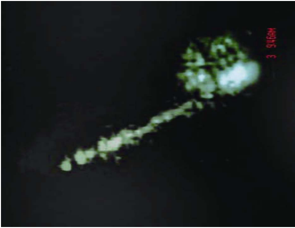
Fig. 4. The image of SAMHO BROTHER sunk at the depth of 70 m. The side scan taken by R/V Ocean Researcher 2 of National Taiwan Ocean University. (25/10/2005, R/V OR2)
