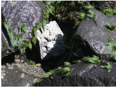
Fig. 4. Natural culture of the marine algae U. fasciata on concrete cube.
