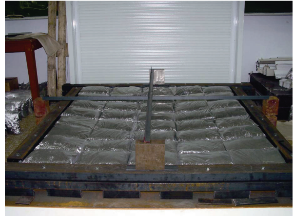
Fig. 9. Deformation test of a shutter assembly loaded by uniformly distributed sand bags.
