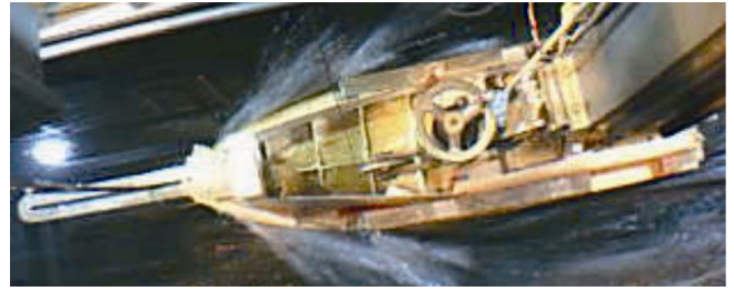
Fig. 7. A photo of wave patterns around the model during experiment in the towing tank.
