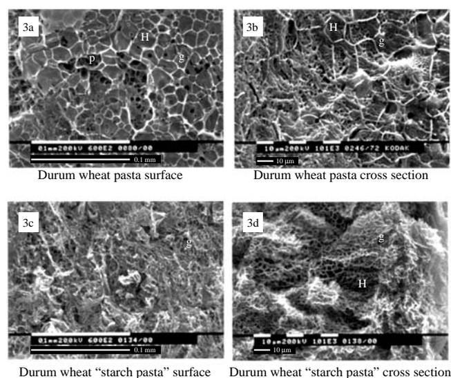
Fig. 3. Freeze dried pasta and starch pasta after 5 minutes cooking. H) Honeycomb-like structure; p) porous network; g) gelatinized starch.
