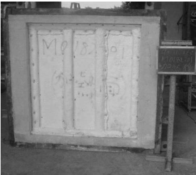
Fig. 12. No damage surface of ceramic fiber after the 60 minutes fire test.
