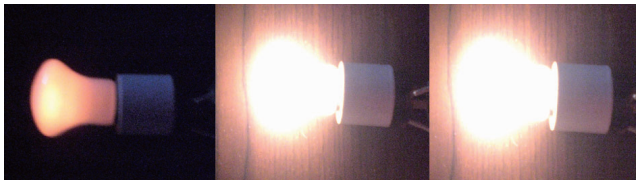
Fig. 14. Bulb responses for control value DN = 5, 15, 25.
