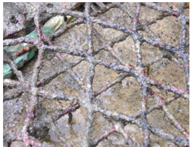
Fig. 12. The appearance of conductive rubber coatings (CR-P-N) after 500 days in the field test.
