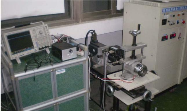
Fig. 14. The dynamometer test bench.
