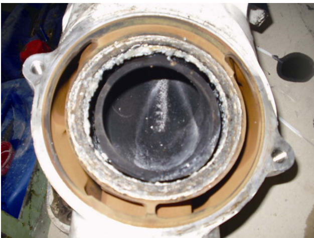
Fig. 6. Sea salt, mildew and less rusting before the turbocharger inlet.
