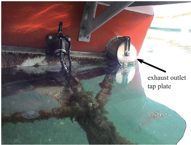
Fig. 3. External view of the ransom stern and the exhaust outlet.
