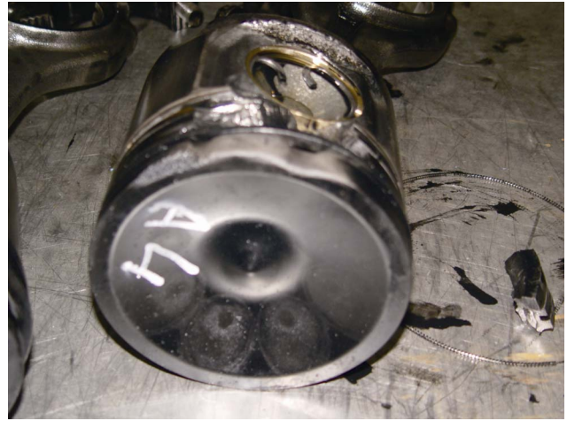
Fig. 10. Pitting and sea salt contours on piston crown.
