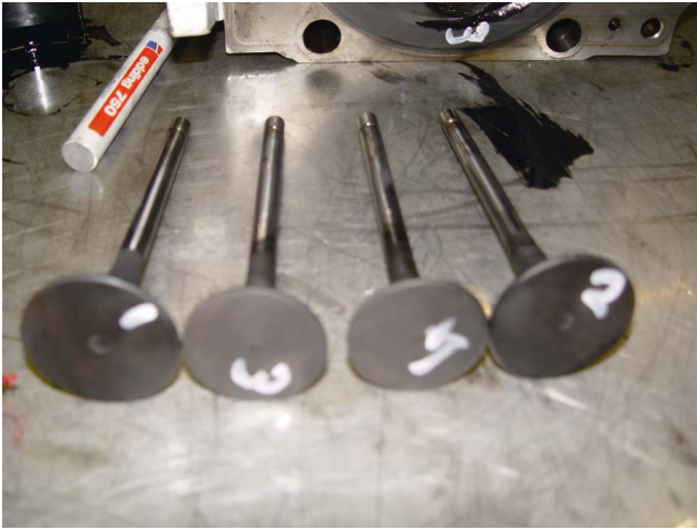
Fig. 9. Less evidence of rusting on the exhaust valve skirts.
