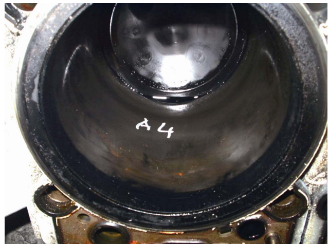
Fig. 8. Local rusting on the liner's inner surface.
