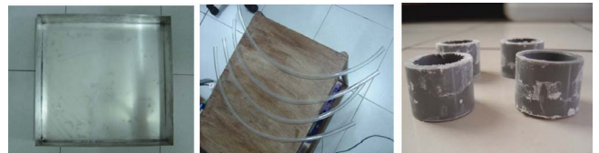
Fig. 6. Aluminum metal box and plastic tubing used in simulation experiment.
