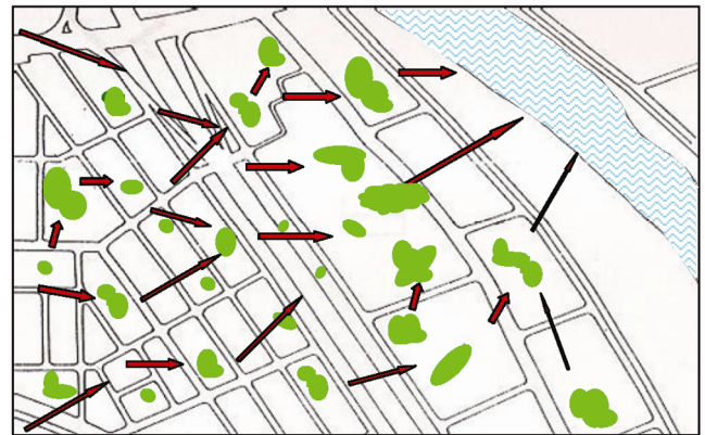
Fig. 7. Schematic diagram of scattered low-impact runoff retardation facilities [1].
