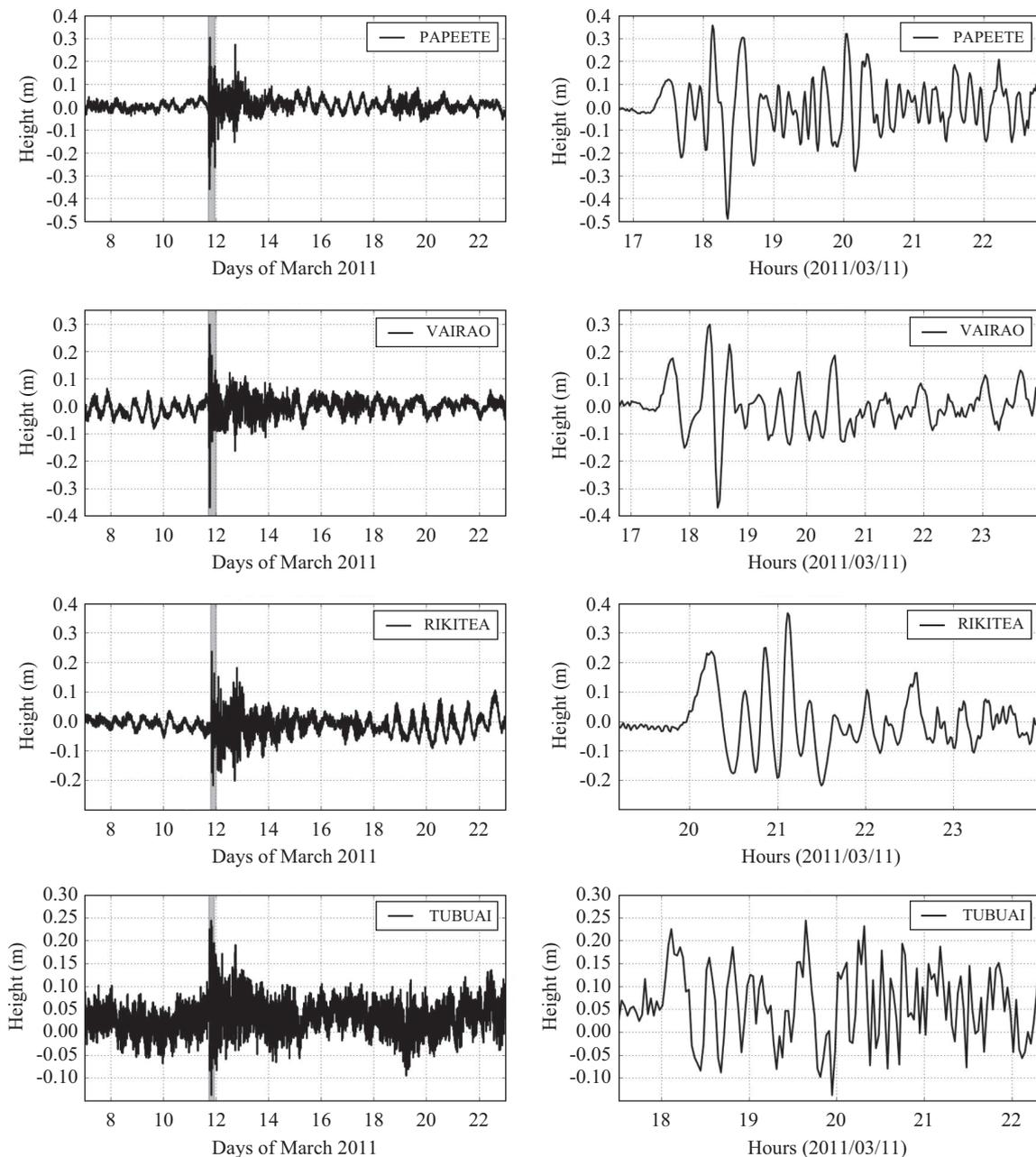
Fig. 4-b. Filtered tsunami signals (left) for the March 11, 2011 tsunami event for the tide gauges of Papeete, Vairao, Rikitea and Tubuai. Enlargements of the greyed areas are shown in the right figures (a few hours window after the arrival of the first wave).
