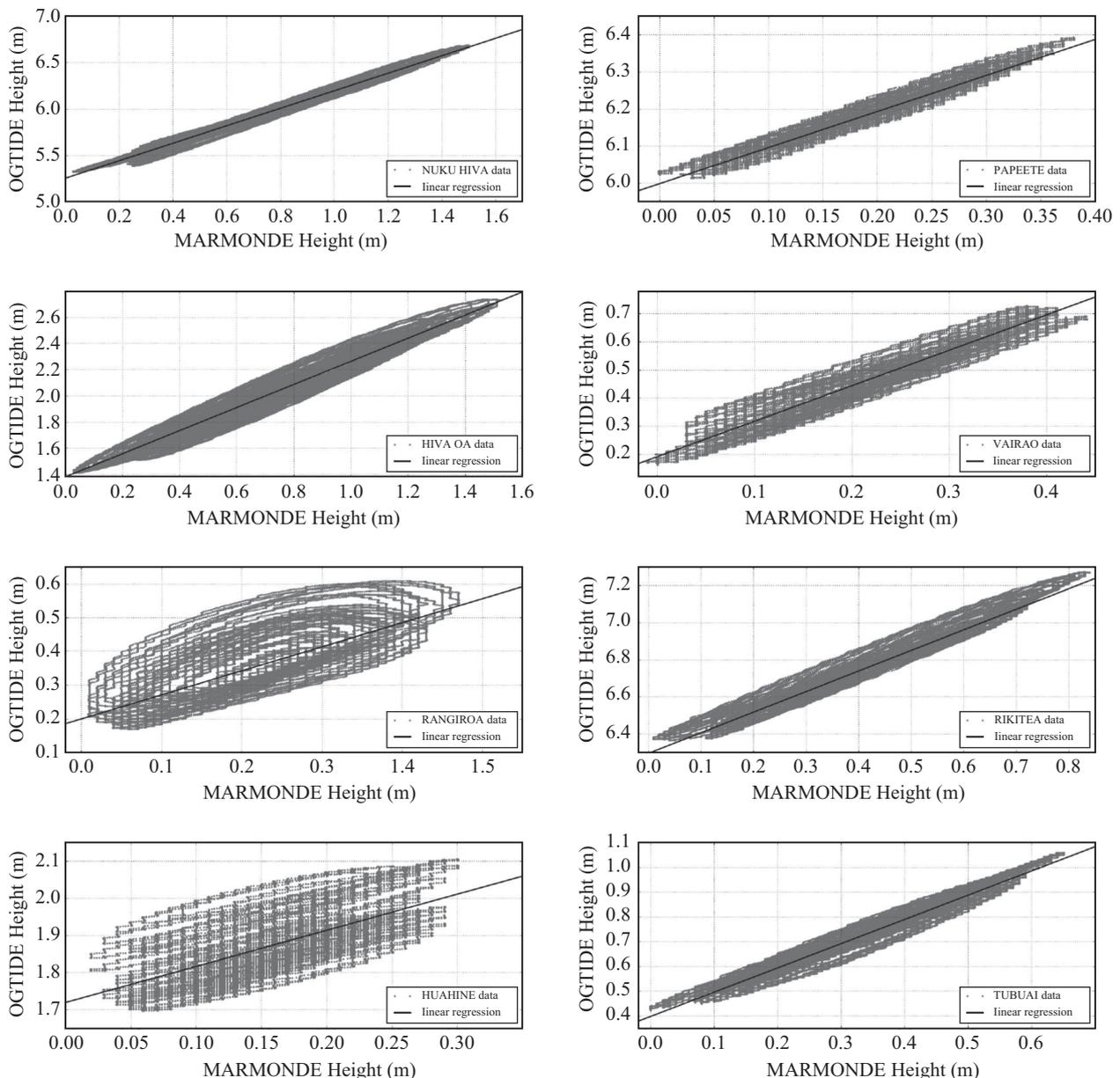
**Fig. 3.** Least-squares analysis of the tides computed by MARMONDE model (SHOM) with respect to the M4, MS4, S4, M6, M2, S2, N2, K2, O1, K1, P1, Q1, MF and MM harmonic constituents of the oceanic tides (see text). Notice the large phase delays for the tide gauges of Huahine and Rangiroa, and, to a lesser extent, Vairao.
