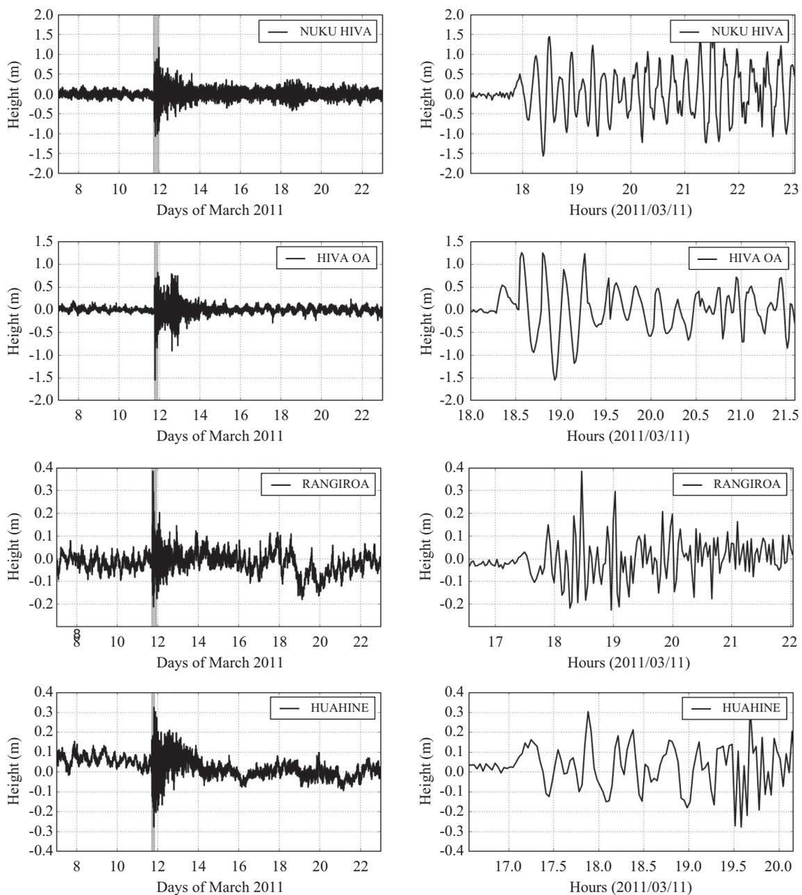
**Fig. 4-a. Filtered tsunami signals (left) for the March 11, 2011 tsunami event for the tide gauges of Nuku Hiva, Hiva Oa, Rangiroa and Huahine. Enlargements of the greyed areas are shown in the right figures (a few hours window after the arrival of the first wave).**
