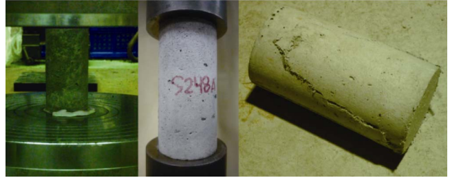
Fig. 2. ECC compression test.
