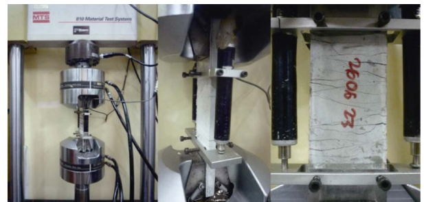
Fig. 4. ECC tensile test setup.
