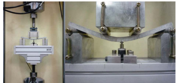
Fig. 3. ECC flexural test setup.
