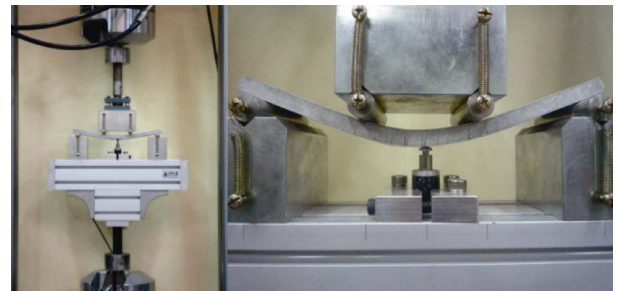
Fig. 3. ECC flexural test setup.
