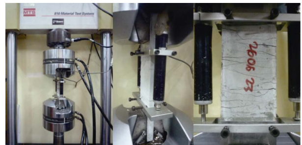
Fig. 4. ECC tensile test setup.
