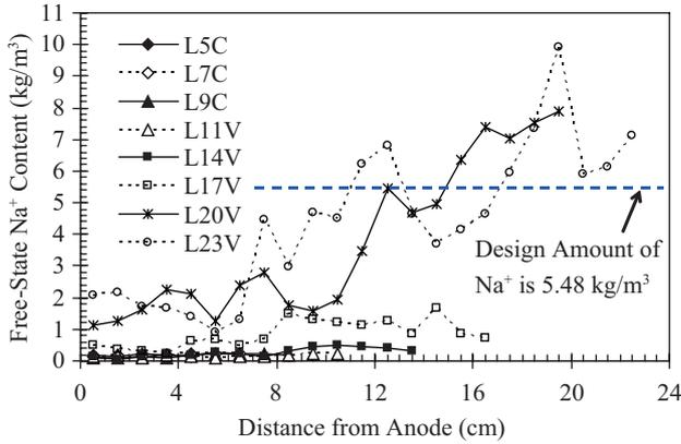
Fig. 12. Free-state Na<sup>+</sup> content inside specimen after electrolysis.
