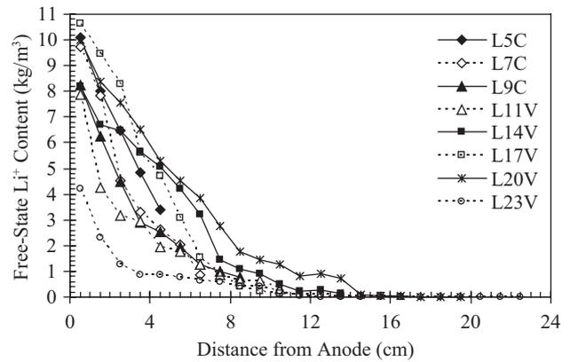
Fig. 11. Free-state  $Li^+$  content inside specimen after electrolysis.
