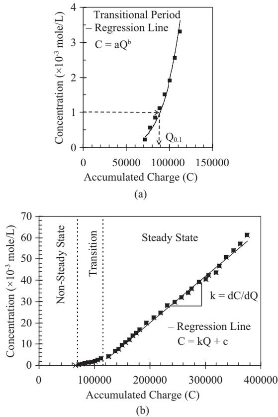
**Fig. 8. Changes of Li<sup>+</sup> concentration in the catholyte (using Experiment L9C as an example).**
