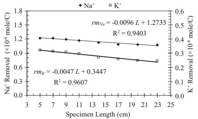
**Fig. 5. Relationship between Na<sup>+</sup> and K<sup>+</sup> removal amount per unit charge during steady migration ( $rm_{Na}$  and  $rm_K$ ) and specimen length.**
