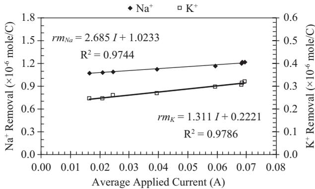
Fig. 6. Relationship between Na<sup>+</sup> and K<sup>+</sup> removal amount per unit charge during steady migration ( $rm_{Na}$  and  $rm_K$ ) and average applied current ( $I$ ).
