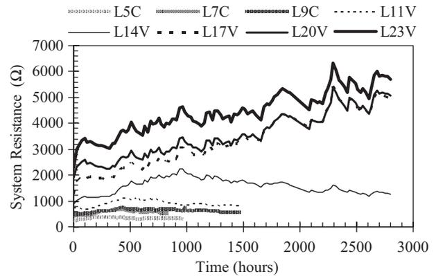
Fig. 2. System resistance during the duration of electrolysis.
