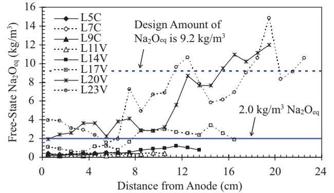
Fig. 14. Free-state Na<sub>2</sub>O<sub>eq</sub> content inside specimen after electrolysis.
