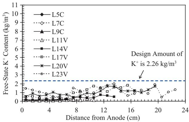
Fig. 13. Free-state K<sup>+</sup> content inside specimen after electrolysis.
