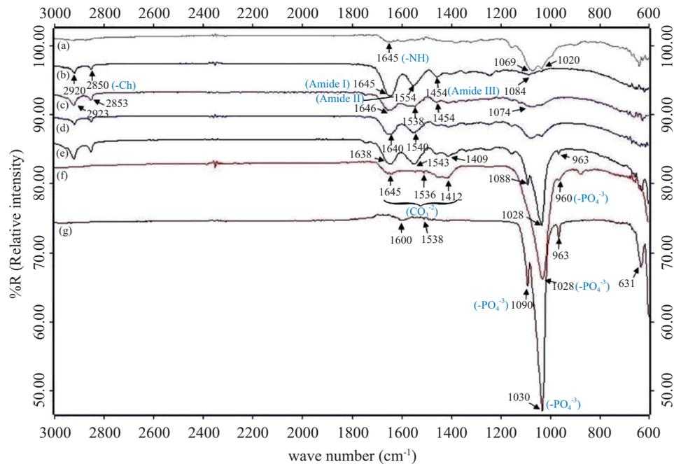
Fig. 1. ATR-FTIR spectra of (a) Chitosan, (b) Gelatin, (c) CS/GEL, (d) CS/GEL/FHAP, (e) CS/GEL/sFHAP, (f) FHAP, and (g) sFHAP.
