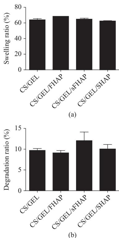
Fig. 3. (a) Swelling behavior and (b) degradation behavior of CS/GEL/hydroxyapatite membranes.
