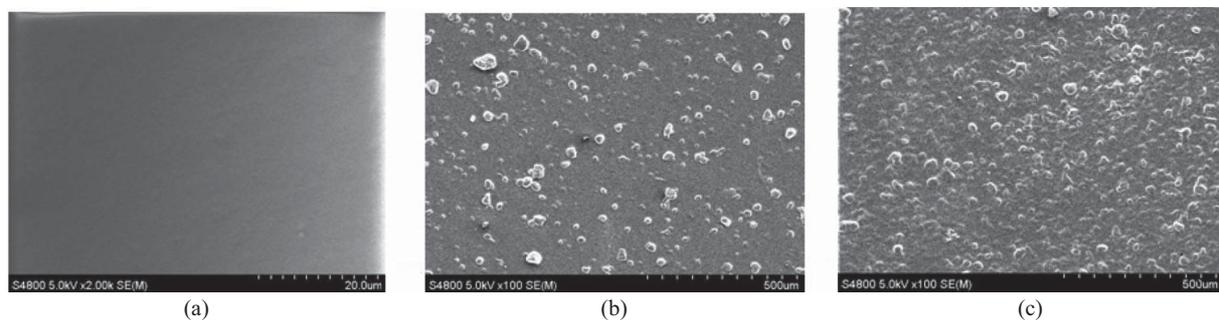
Fig. 2. SEM micrographs of CS/GEL/FHAP membrane before (b) and after (c) sintering. The CS/GEL membrane (as a control) is shown in the image (a).
