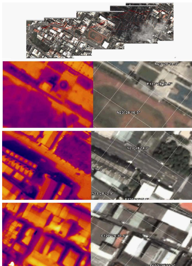
Fig. 2. Examples of images acquired by the helicopter-borne IR Imager (red-blue images). The right panels correspond to the high resolution satellite images (true color images) from the Google map.
