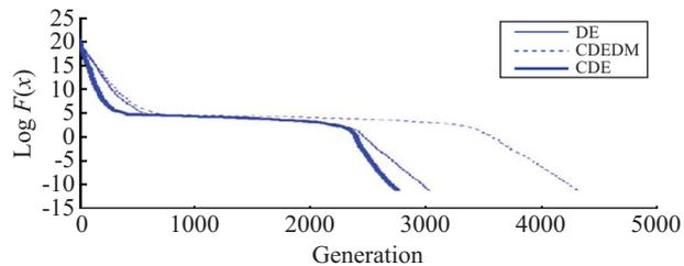
Fig. 10. Convergence process of the objective function value of  $f_3$ .
