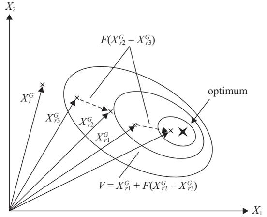
Fig. 1. The generation of a trial vector in a mutation [22].
