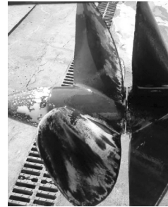
Fig. 27. Aluminum propellers corrosion.
