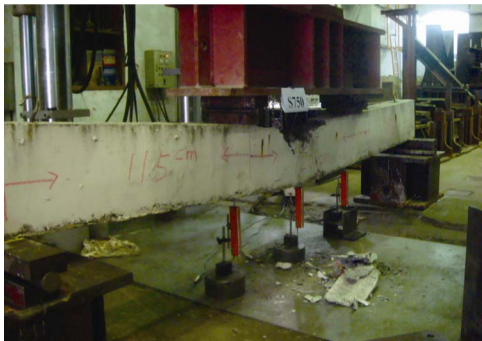
Fig. 4. P-A loading test.
