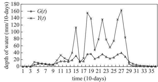
**Fig. 6. Simulated drainage discharge and downward percolation.**
