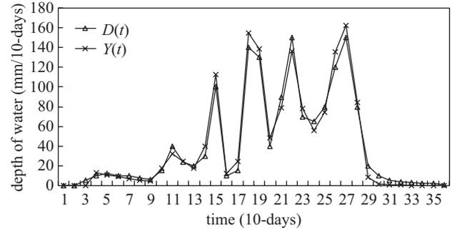
**Fig. 5. Simulated and actual drainage discharge.**
