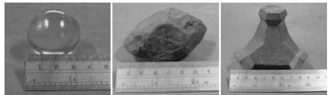
Fig. 2. Three materials of the porous submerged breakwater. From left to right are the glass bead, the rubble rock, and the armor unit, respectively.
