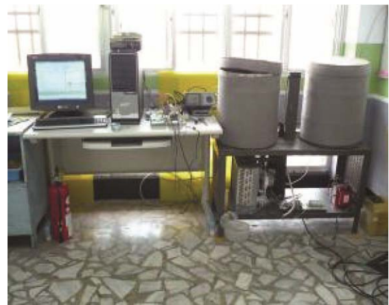
Fig. 12. Hardware for the intelligent heat pump heater.
