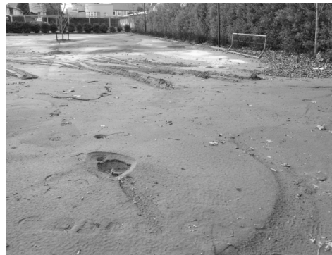
Fig. 2. Silty sand liquefaction at central business district of Christchurch during 2010-2011 Christchurch Earthquakes, New Zealand.
