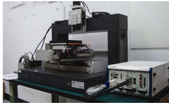
Fig. 12. The PMLSM positioning platform system.
