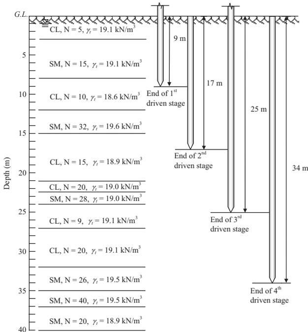
Fig. 4. Subsoil condition and processes of a pile being driven into subsoil of the Chiayi-Taibao City (Redrawn from Hwang *et al.* [18]).
