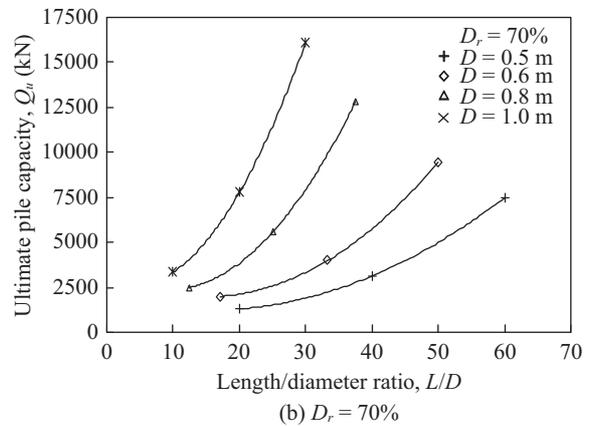
Fig. 13. Relationships between the ultimate pile capacity and length/diameter ratio  $L/D$  for various pile diameters and various relative densities of silty sand.
