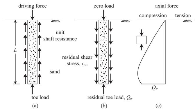
Fig. 1. Residual load induced by driving a pile (Alawneh *et al.* [1]).
