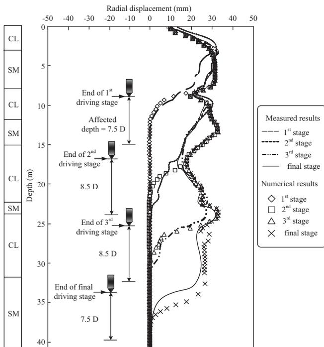
**Fig. 7. Comparison of measured and modeled radial ground movement at a distance of  $3D$  (2.4 m) from the center of the pile (Note: the measured results were redrawn from Hwang *et al.* [18]).**
