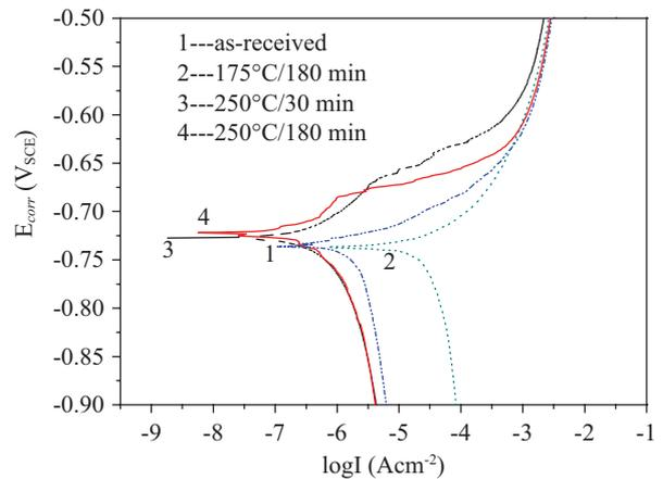
Fig. 4. Potentiodynamic polarization curves for the naturally exfoliated 5456-H116 alloy annealed at 175°C for 180 minutes and at 250°C for two time periods: 30 and 180 minutes (measured in 3.5% NaCl solution, scanning rate is 5 mV/s).
