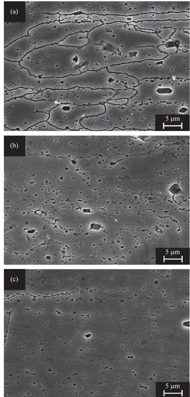
**Fig. 6.** SEM micrograph showing the effect of stabilization heat treatment on the microstructure of the as-received specimen and specimens annealed at 250°C for different lengths of time: (a) as-received, (b) 10 minutes, (c) 30 minutes.
