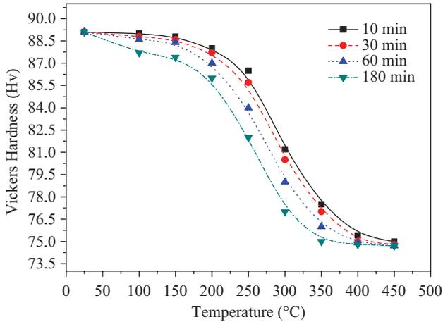
Fig. 2. Variation of hardness with heat treatment conditions for the naturally exfoliated 5456-H116 plate.
