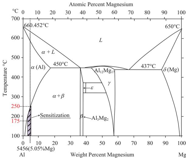
Fig. 1. Phase diagram of the Al-Mg binary system with the composition of marine-grade alloys sensitization region indicated [12].
