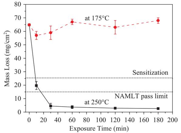
Fig. 3. NAMLT test (immersion into HNO<sub>3</sub> for 24 h) results of the 5456-H116 samples after being treated in the stabilization and sensitizing temperature for 10, 30, 60, 120, and 180 minutes.
