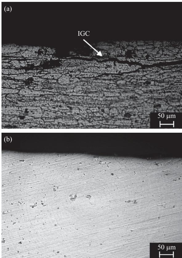
Fig. 7. Optical micrographs of the naturally exfoliated 5456-H116 specimens: (a) as-received, and (b) heat-treated at 250°C for 30 minutes, and then immersed in 70% HNO<sub>3</sub> for 24 h.
