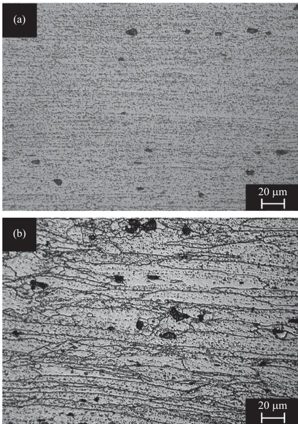
**Fig. 5.** Microstructures with variations in continuity of matrix grain boundary and  $\beta$  precipitation: (a) unsensitized 5456-H116, showing undetectable grain boundary, (b) naturally exfoliated 5456-H116, showing continuous network of grain boundary.
