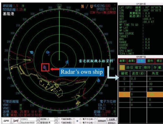
Fig. 15. A snapshot of MAST's screen. Five targets are created. Target#0 is chosen as the own ship for the radar simulator.
