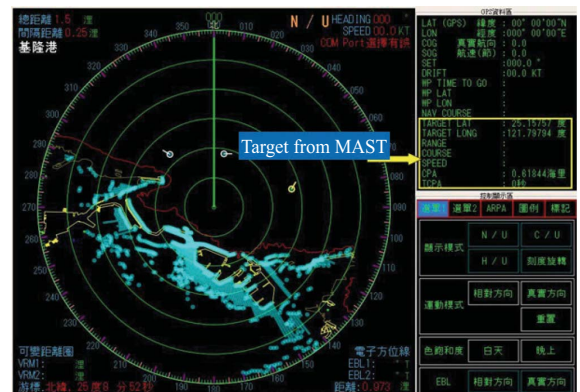
Fig. 16. A snapshot of the radar simulator fed with targets and own ship data from the connected MAST.
