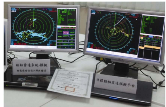
Fig. 17. Demonstration of a radar simulator (left) connected with a multi-agent ship traffic simulation platform (right), operated on laptop PCs.
