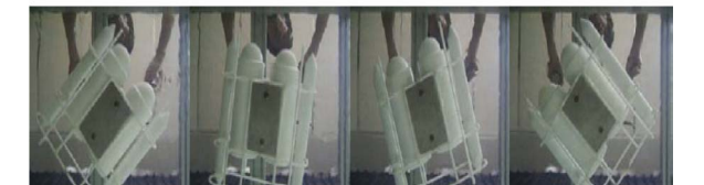
Fig. 17. Image sequence of the scale model in the yaw direction [4].
