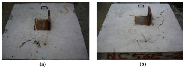
Fig. 13. The failure patterns of the bearing type (56E) specimen for shearing test after the fire resistance test (a) specimen LC(56E)V2b (b) specimen NC(56E)V2b.
