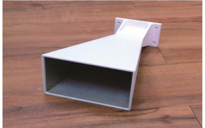
**Fig. 5. Photograph of the Prototype pyramidal horn antenna.**
