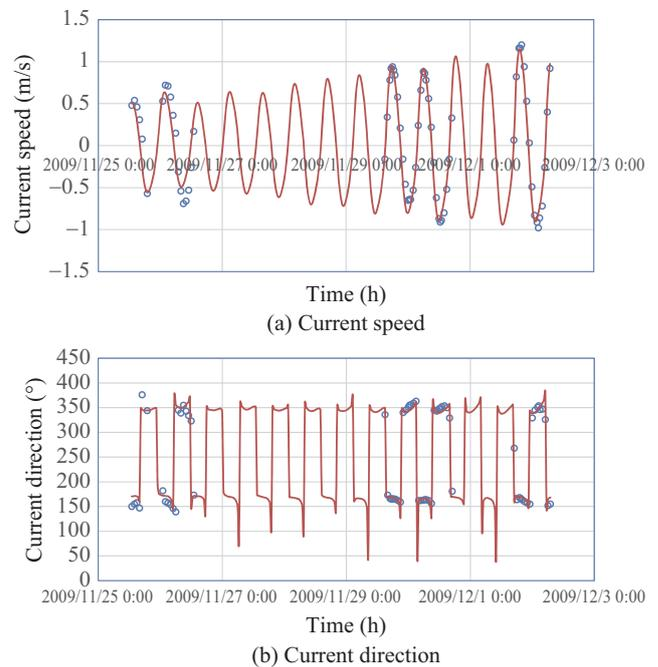
**Fig. 6. Comparisons of simulated and measured depth-averaged current at P<sub>6</sub> station.**
