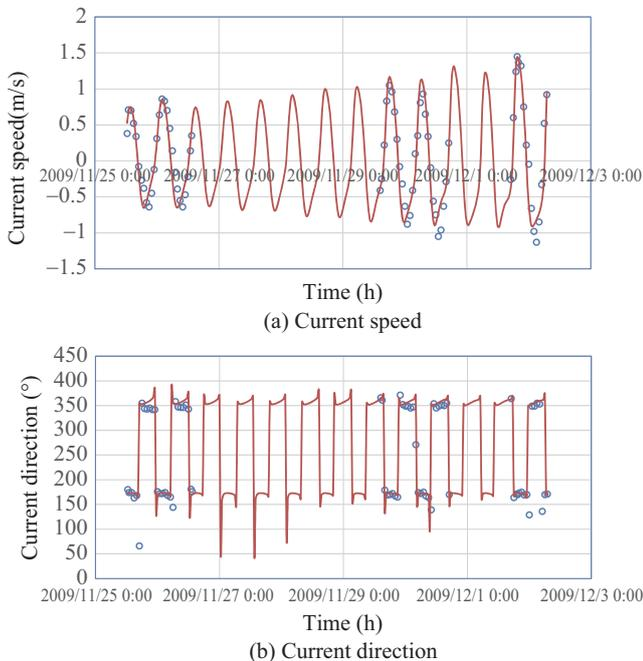
**Fig. 4. Comparisons of simulated and measured depth-averaged current at P<sub>2</sub> station.**
