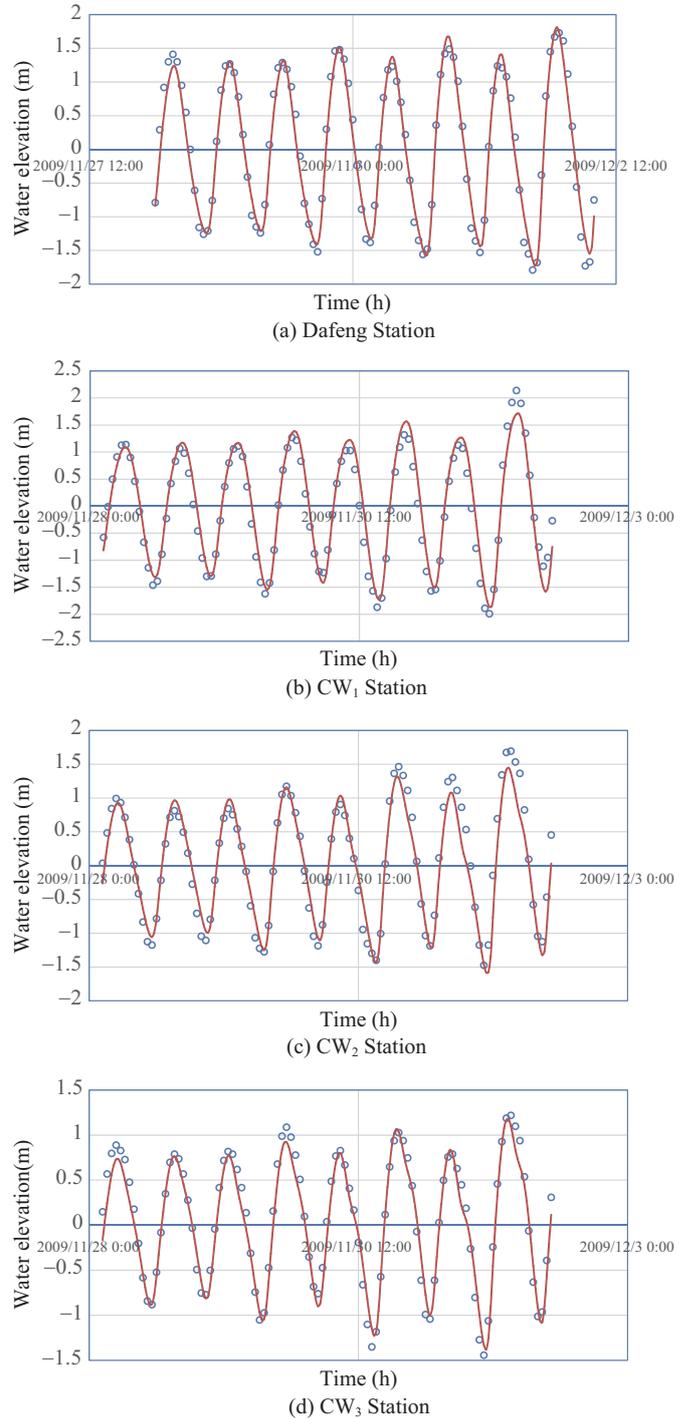
Fig. 2. Comparisons of simulated water elevation and measured data.
