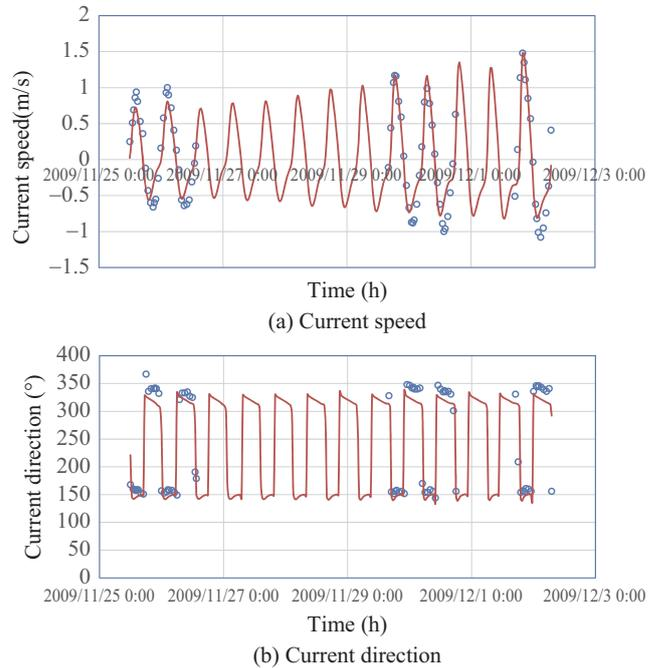
**Fig. 5. Comparisons of simulated and measured depth-averaged current at P<sub>4</sub> station.**
