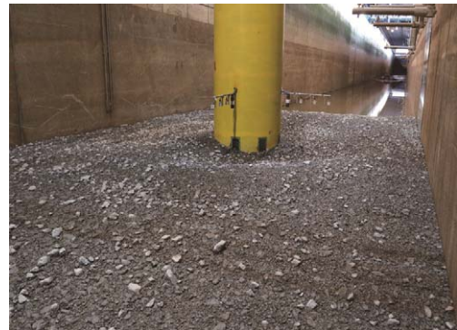
Fig. 4. Final scour development around the monopile after 9000 waves and maximum significant wave height H_s = 1.3 m. Waves are propagation in viewing direction.
