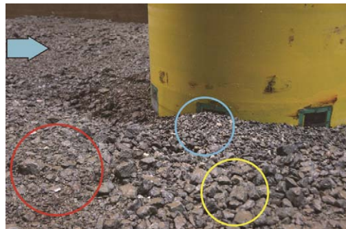
Fig. 5. Tendencies of an armour layer development (red circle), deposition of finer fractions on the sides (blue circle) and coarser fractions (yellow circle) around the monopile after 3000 waves with H_s = 0.7 m. Waves are coming from the left side.
