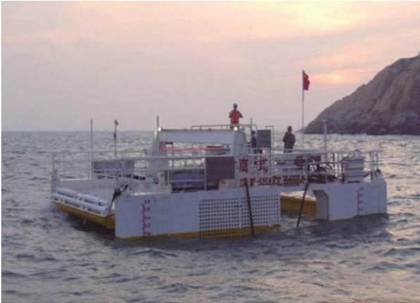
Fig. 5. The 10 kW Eagle WEC developed by GIEC.
