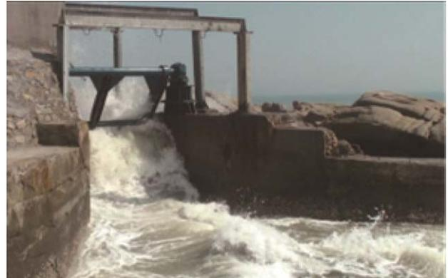
Fig. 3. The 30 kW pendulum WEC developed by NOTC.
