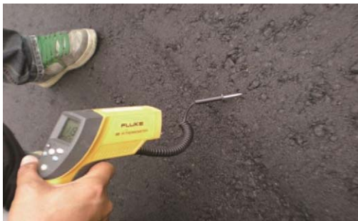
Fig. 3. Detecting with infrared temperature-sensing gun.
