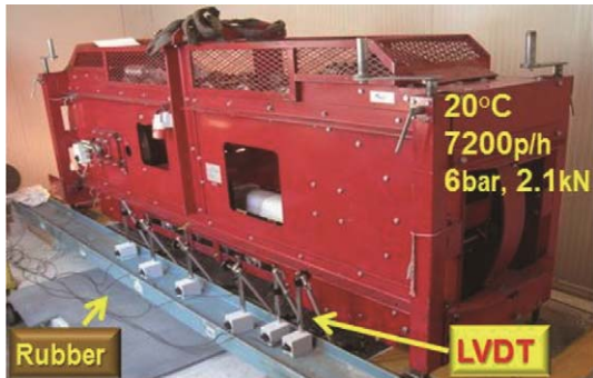
Fig. 10. MMLS3 with deformation sensors.
