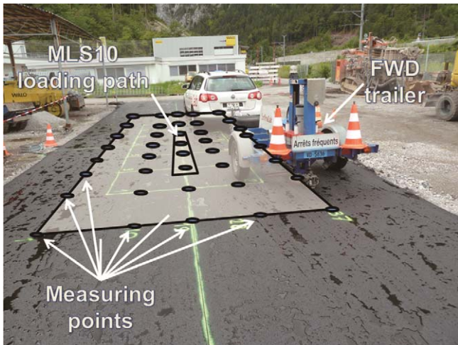
Fig. 22. View of the Falling Weight Deflectometer (FWD) in testing position.
