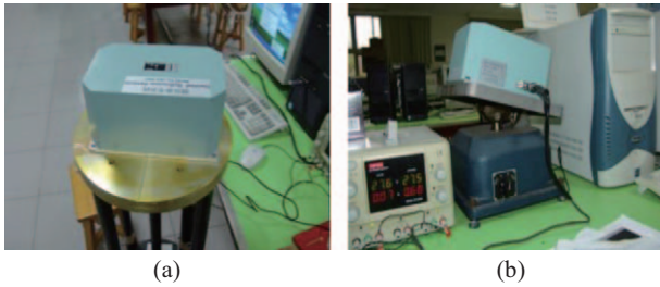
Fig. 6. INS system test equipments (a) static test conducted on a horizontal rotation table, and (b) dynamic test conducted on a Scorsby motion test platform, which is derived by single shaft, rotating in a cone.
