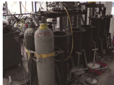
Fig. 2. Accelerated carbonation equipment.
