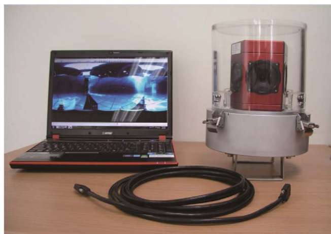
Fig. 3. Undersea panoramic photography equipment included a laptop, spherical digital video camera, cylindrical waterproof housing, and IEEE-1394b cable.
