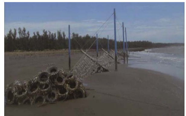
Fig. 7. The No. 1 flexible device and appearance of the beach after a typhoon on 2009/07/04, one month after the device was set-up. Rich sediment is deposited around the device. The bottom row of the flexible net (attached with tires) was buried by sediment.
